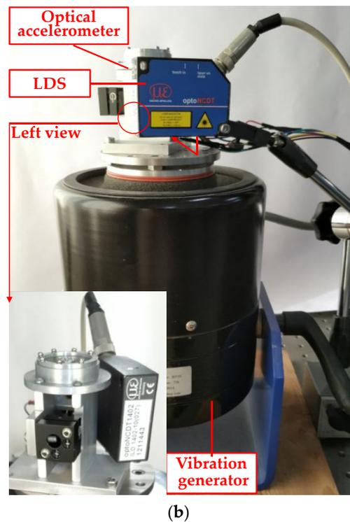
**Figure 6.** Experimental setup for the designed optical accelerometer calibration. (a) Diagram, (b) photo. LDS: laser displacement sensor.
