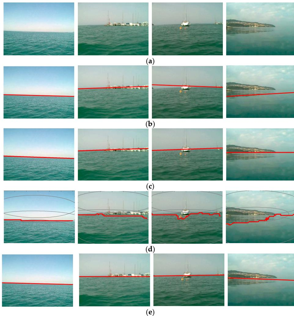
**Figure 12.** A comparison of various horizon line detection methods using MODD: (a) Original image; (b) Wang's algorithm; (c) MSCM-LiFe; (d) SSM; (e) CFS method.
