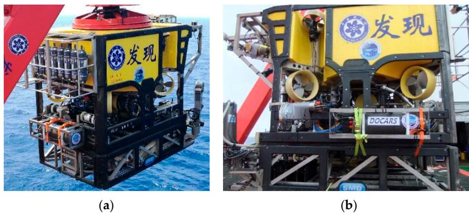
**Figure 2.** ROV installation solutions for DOCARS system. (a) Back mounting case. (b) Side mounting case.
