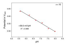
**Figure 6.** Influence of pH value: Measurement in air-saturated electrolyte with different pH. Potential is plotted with respect to normal hydrogen electrode (NHE).
