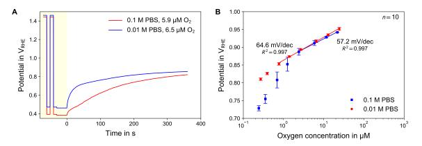
Figure 5. Influence of the ion-strength of the electrolyte: Comparison of time trace (A) for concentration with same oxygen fraction in gas phase and calibration curves (B) using a duration of 360 s for the OCP phase.
