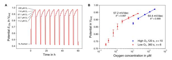
**Figure 4.** (**A**) Trace of active potentiometry measurements of 10 consecutive concentration ramps with higher oxygen concentrations. (**B**) Calibration curves for the concentrations ramp with higher and lower oxygen concentration range. In case of lower oxygen concentrations (red disks) the OCP phase was prolonged to 360 s.
