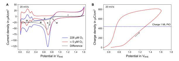
**Figure 2.** (**A**) Cyclic voltammograms (CV) of platinum in air-saturated (dashed curve) and nitrogen flushed (dotted curve) in 0.1 M PBS. The difference signal (solid curve) is assumed to represent mainly the oxygen reduction process at platinum. (**B**) Charge (integral of the current in A) for the nitrogen flushed CV in the region of platinum oxide formation. The dashed line represents the charge needed to form 1 monolayer (ML) of PtO.
