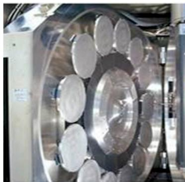
**Figure 1.** The rotating disk and wafer holders in the batch type ion implanters (courtesy of SMIT).
