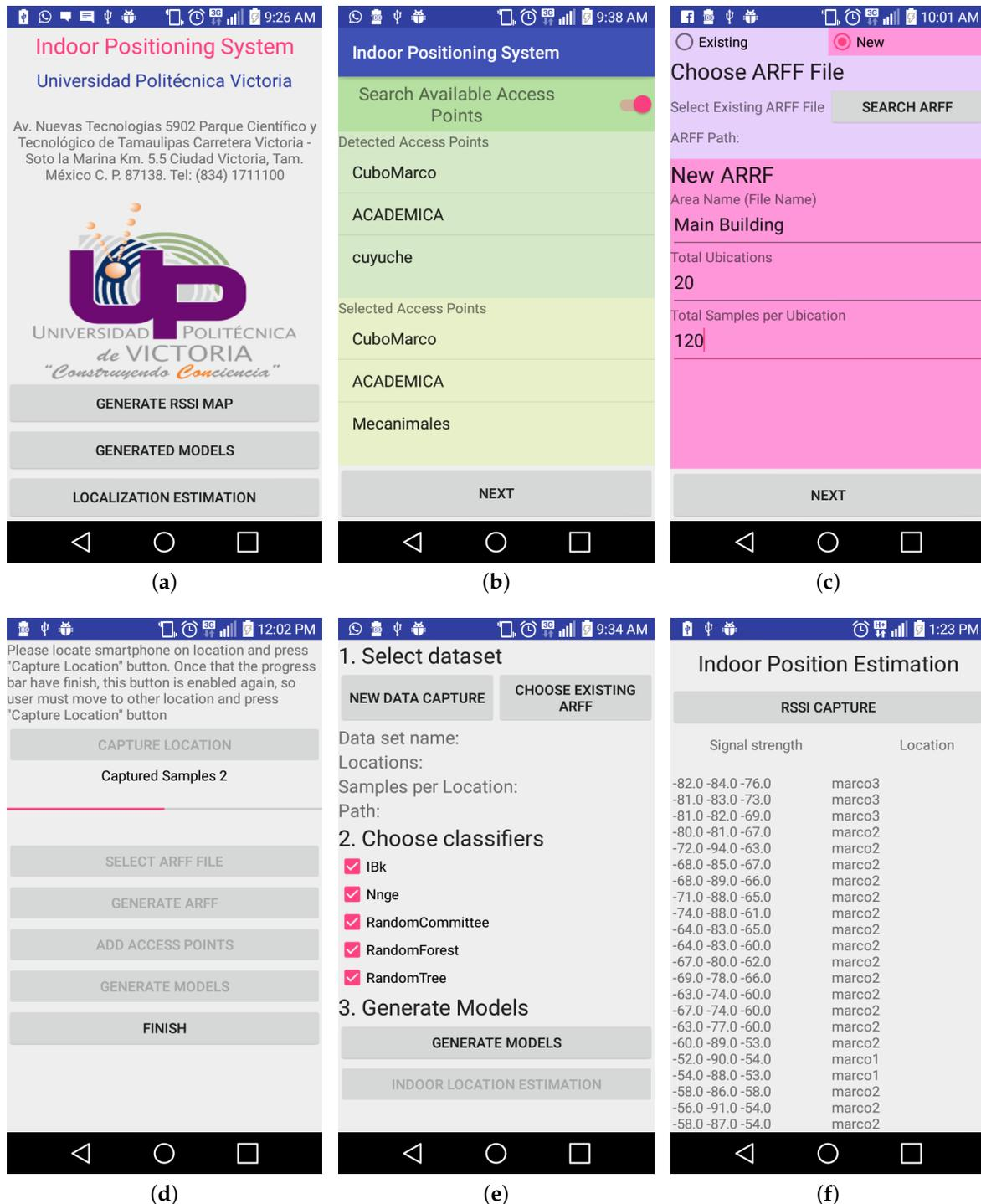
**Figure 3.** Screen of the proposed IPMApp application. (a) Main screen; (b) Access point selection; (c) Configuration of captured dataset; (d) RSSI signal capture; (e) Training of ML classifiers; (f) Real-time indoor position estimation.
