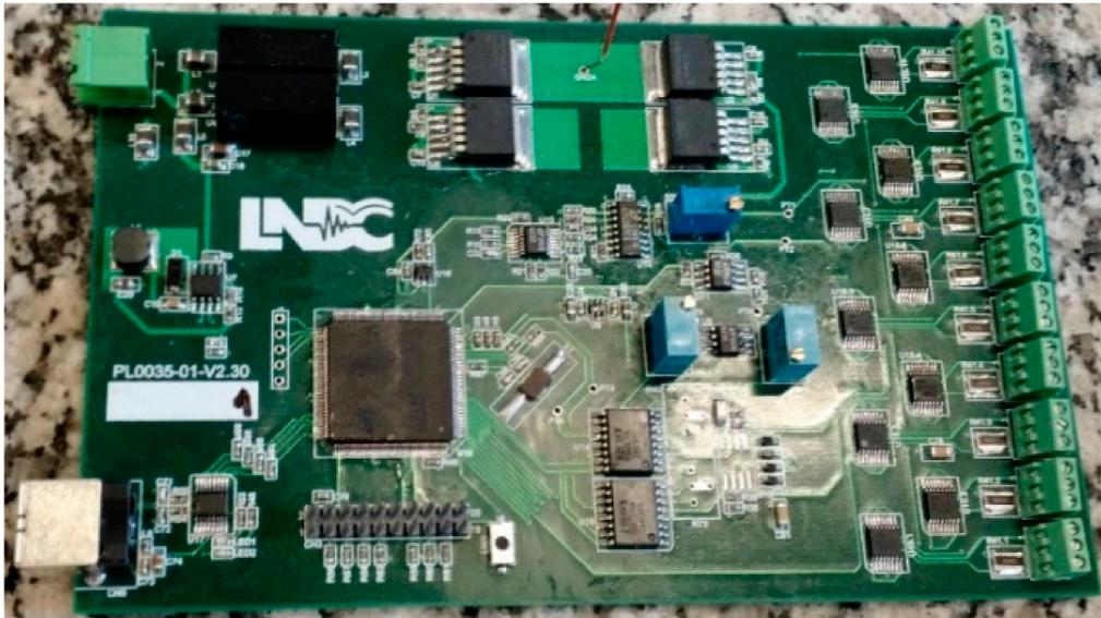
**Figure 7.** Photo of the electronic hardware developed to drive and measure the EC transducer impedance variation.
