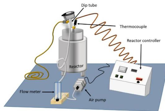
**Figure 1.** Equipment used to thermally oxidize engine oil.
