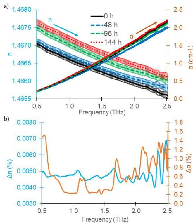
**Figure 3.** (a) Mean refractive index (left axis) and mean absorption coefficient (right axis) of gasoline engine oil (5W20) oxidized over four different times from three measurements of the 15 mm cuvette of gasoline engine oil with 95% confidence interval bars; (b) Relative values for the CI of the refractive index (left axis) and absorption coefficient (right axis).
