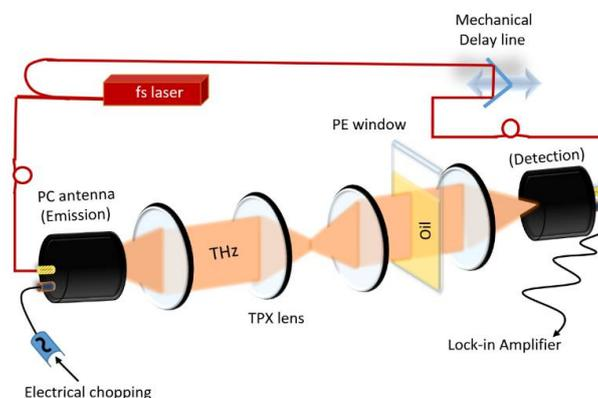
**Figure 2.** Depiction of a THz time-domain spectrometer.
