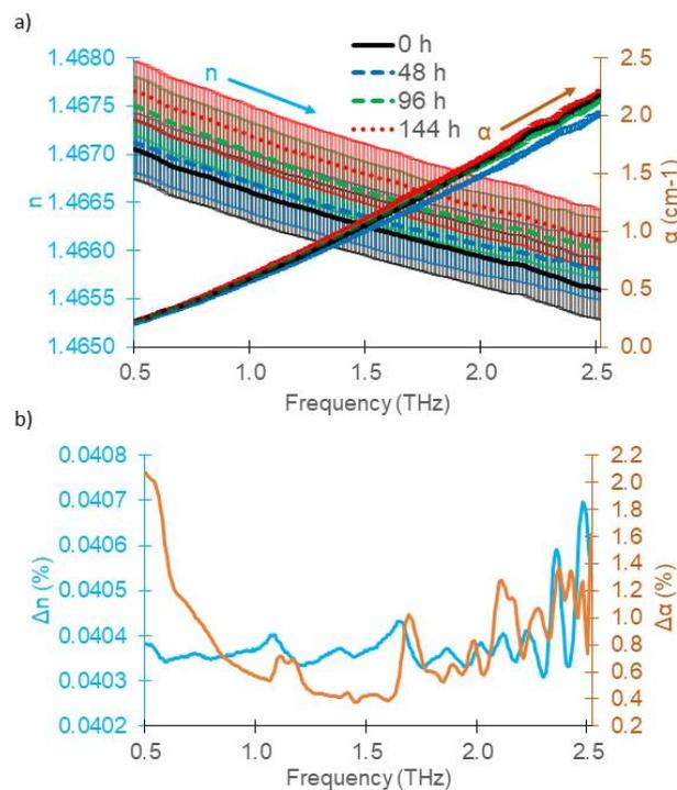
**Figure 4.** (a) Mean refractive index and absorption coefficient of gasoline engine oil (5W20) oxidized over four different times from three measurements of the 15 mm cuvette; (b) 95% confidence intervals for  $n$  and  $\alpha$ , taking the CI of the probe volume thickness into account.
