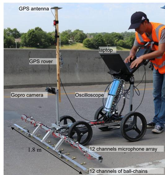
**Figure 1.** 12-channel acoustic scanning cart.
