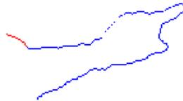
**Figure 5.** Pixels on the perimeter of an arm segment and adjacent to the rest of the foreground (binary image  $B_{inner}$ , also shown in Figure 4). The pixels used to connect graph layers (binary image  $B_{connect}$ ) are shown in red.
