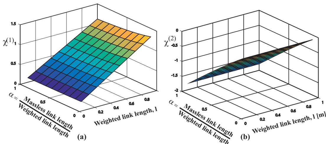
**Figure 15.** Mode ratio results: first mode  $1.5 \geq \chi^{(1)} > 0$  both links swing in nearly in phase; second mode  $0 > \chi^{(2)} > -2$  both links swing in opposite phases. Conditions:  $l \leq 1$  m,  $0 < \alpha \leq 1$ .
