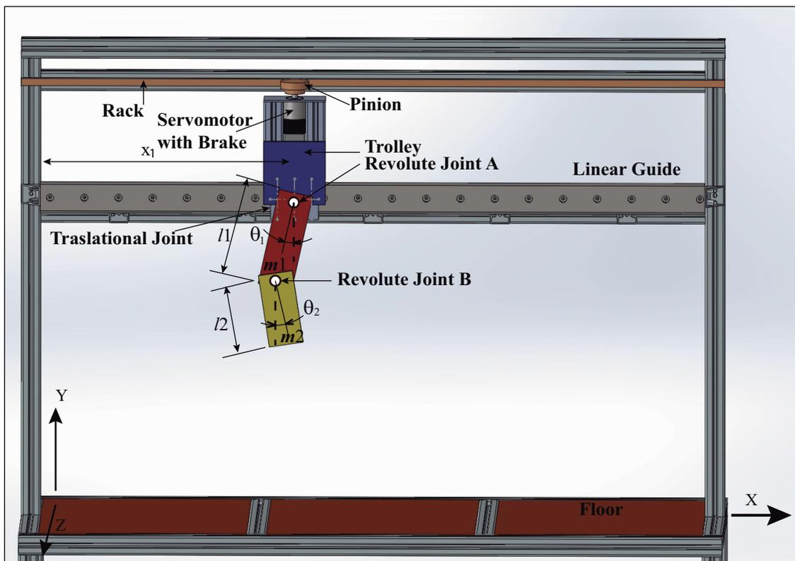
**Figure 6.** Sketch of the overhead crane Functional Mock-Up Interface (FMI) with double pendulum multibody payload dynamics. Conditions: first link, length  $l_1$ , mass  $m_1$ , plus moment of inertia about the mass center  $I_{zz}^{G1}$ ; second link, length  $l_2$ , mass  $m_2$ , plus moment of inertia about the mass center  $I_{zz}^{G2}$ .
