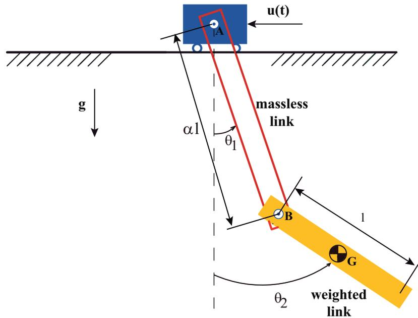
**Figure 13.** Planar double pendulum. Conditions: massless first link length  $\alpha \cdot l$  equivalence with composite revolute-revolute joint and the weighted second link with mass  $m$ , plus moment of inertia about the mass center  $I_{zz}^G$ .
