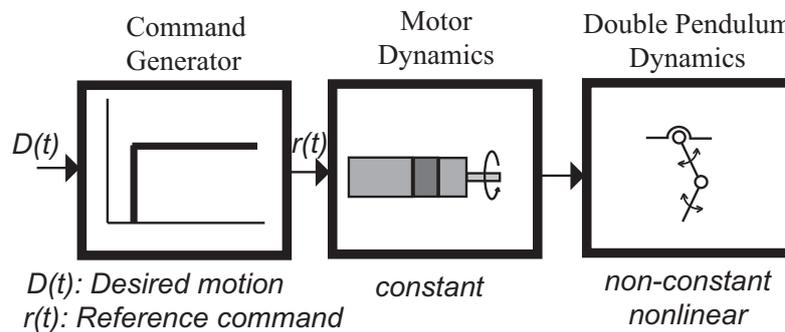
Figure 17. Block diagram of the generic control system.
