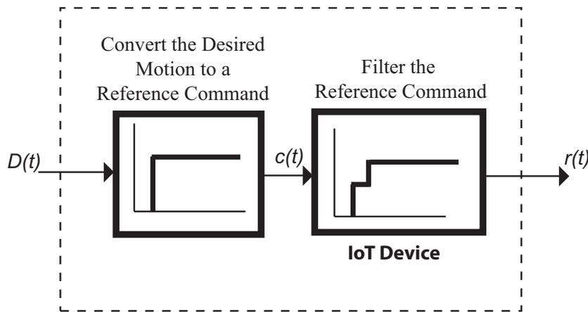
Figure 18. Command generator for real-time command shaping.
