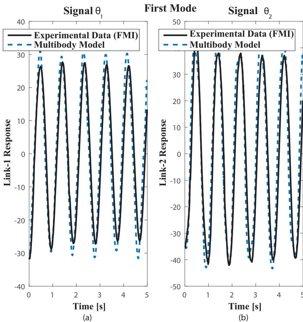
**Figure 7.** Plots of Experimental FMI and Multibody model free vibration motion responses closely to the first mode. Initial Conditions: first link deviation from vertical  $\Theta_1 = 31.84^\circ$ , clockwise, second link deviation from vertical  $\Theta_2 = 26.39^\circ$ , clockwise.
