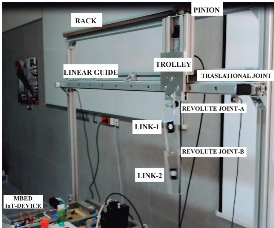
**Figure 24.** Mini Overhead Crane functional mock-up interface.
