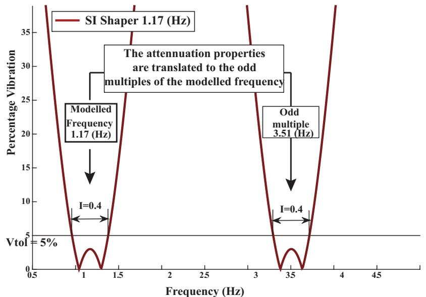
Figure 20. SI Shaper 1.17 Hz sensitivity curve.
