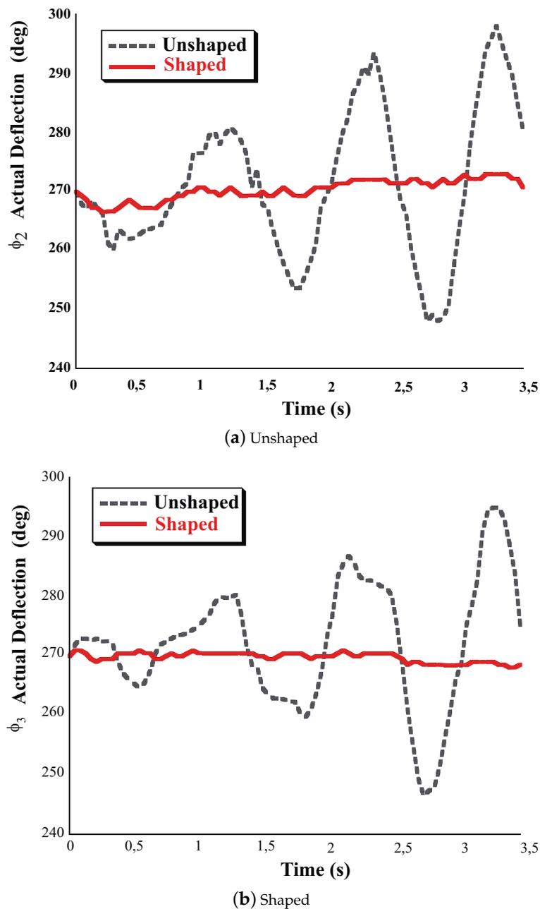
**Figure 26.** Unshaped and Direct SI-Shaped Experimental Responses of the Hydraulic crane under slewing motion. Conditions: sampling frequency 60 Hz.
