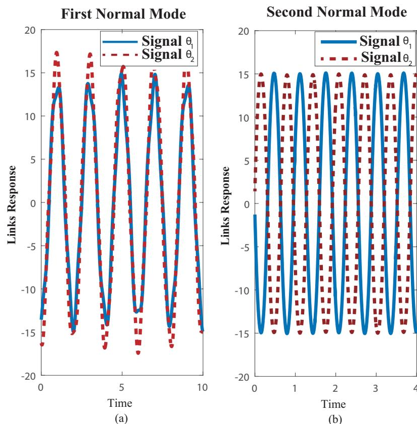
**Figure 16.** Normal Modes of Vibration. First mode both links swing closely in phase; second mode both links swing in opposite phases. Conditions:  $\omega_1 = 0.5$  Hz,  $\omega_2 = 1.86$  Hz,  $\alpha = 0.5833$ ,  $l = 0.8571$  m.
