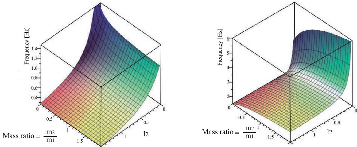
Figure 11. Variation of first and second mode frequencies when  $0 < l_2 < 1.5$  and  $0 < R < 2$ .
