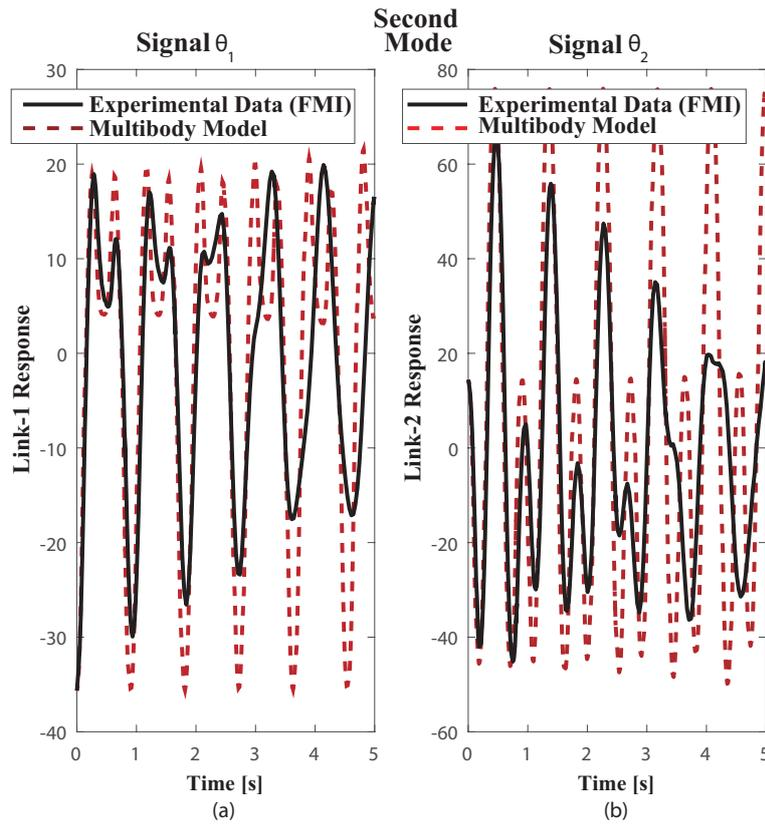
**Figure 8.** Plots of Experimental FMI and Multibody model free vibration motion responses closely to the second mode. Initial Conditions: first link from vertical  $\Theta_1 = 35.65^\circ$ , clockwise, second link from vertical  $\Theta_2 = 14.42^\circ$  counter clockwise.
