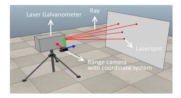
**Figure 4.** Example of calibration setup. The laser rays are described in the laser galvanometer coordinate system. The laser spots are detected and described in the 3D range camera coordinate system.
