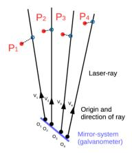
**Figure 3.** Representation of the non-Perspective-n-Point problem with a laser galvanometer. The laser rays ( $O_i$ ,  $V_i$ ) are described in the laser galvanometer coordinate system while laser dots ( $P_i$ ) are described in the range sensor coordinate system.
