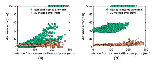
**Figure 11.** Scatter plots with differences between the measured laser spots and the input laser spots in relation with the distance to the center calibration point. "False" values are laser spots that are not detected (out of search range). (a) Distance errors (mm) when the barrel was not moved after 2D calibration. (b) Distance errors (mm) when the barrel was moved 1 m away from the original position.
