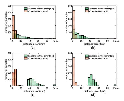
**Figure 10.** Histograms containing the difference between the measured laser spot and the input laser spot. "False" values are laser spots that are not detected (out of search range). (**a**,**b**) Distance errors (pixel, mm) when the barrel was not moved after (2D) calibration. (**c**,**d**) Distance errors (pixel, mm) when the barrel was moved 1 m away from the original position.
