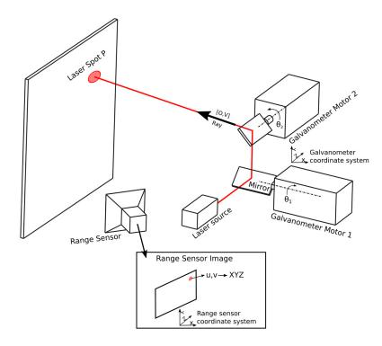
Figure 1. Schematic overview of the galvanometric mirror system and range sensor.
