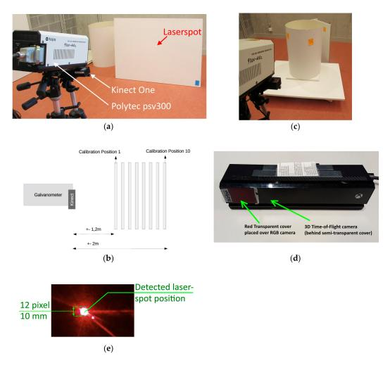
**Figure 6.** (a) Experimental setup for calibrating the system (Polytec PSV 300, Kinect for Xbox One). (b) The calibration plate is moved to different positions. (c) Experimental setup for comparing the 3D calibration with a standard two-dimensional (2D) calibration. (d) Kinect for Xbox One, the RGB camera is covered by a red semitransparent plastic for easier laser spot detection. (e) Result of laser spot detection. The following setup was used to obtain the sample points:
