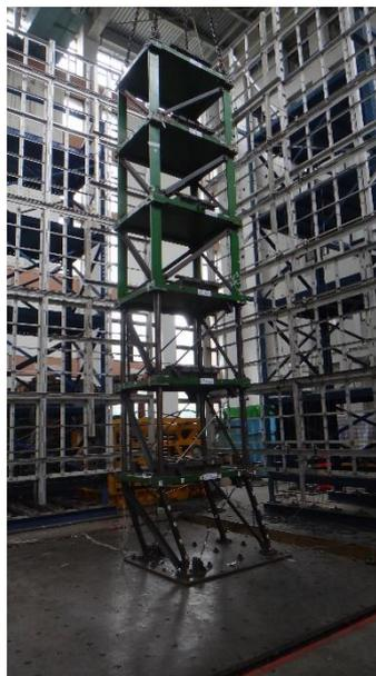
**Figure 7.** A general view of the entire structure in Case 3 after earthquake excitation with a PGA value of 400 Gal.
