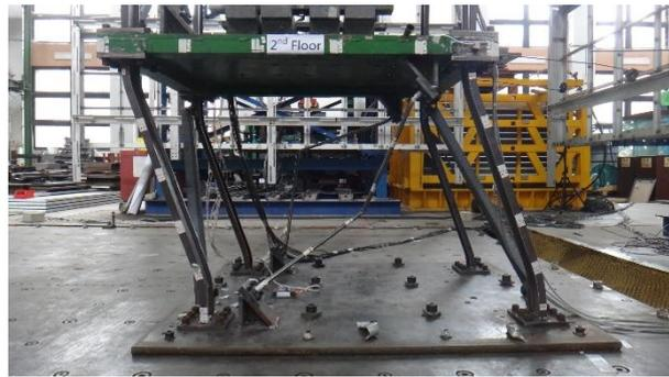
**Figure 6.** A close-up of Story 1 in Case 3 after the earthquake excitation with a PGA value of 400 Gal.
