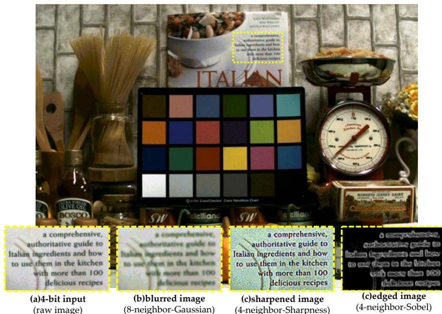
Figure 14. Results of spatial filtering. This is the result of a filter in the yellow area. (a) Raw data; (b) eight-neighbor Gaussian; (c) four-neighbor sharpness; (d) four-neighbor Sobel.
