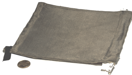
Figure 2. The assembled smart skin with bonded zippers for easier attachment.
