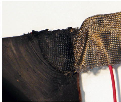
Figure 4. A close-up of CNT PDMS conductive cloth contact detail.
