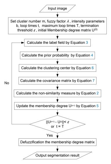
Figure 1. Graphical flowchart of the image segmentation method.
