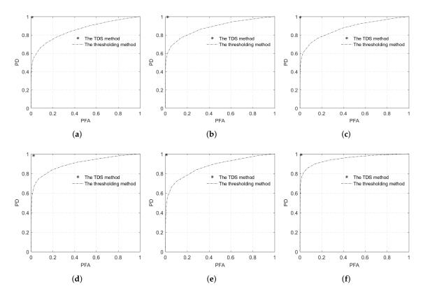
Figure 8. Receiver Operating Characteristic (ROC) curves of the TDS method and the thresholding method.
