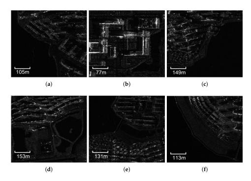
**Figure 3.** The original GF-3 image scenes. (**a**) HH; area: 0.25 km<sup>2</sup>. (**b**) VV; area: 0.14 km<sup>2</sup>. (**c**) HH; area: 0.50 km<sup>2</sup>. (**d**) VV; area: 0.53 km<sup>2</sup>. (**e**) HH; area: 0.39 km<sup>2</sup>. (**f**) HH; area: 0.29 km<sup>2</sup>.
