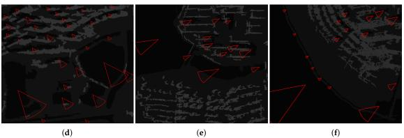
Figure 5. The fan-shape searching strategy from the shadow mass center to the corresponding building (the radius of the fan-shape searching sector is r, and the angle of the fan-shape is  $\theta$ ).
