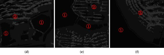
Figure 4. Segmentation results of GF-3 images (① represents water; ② represents building shadow).
