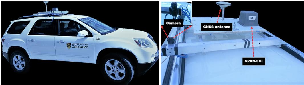
**Figure 13.** Experiment setup. Left: the used vehicle with the mounted equipment; Right: top view of the vehicle.
