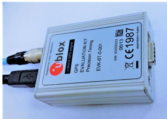
**Figure 12.** The consumer-grade GNSS receiver used.
