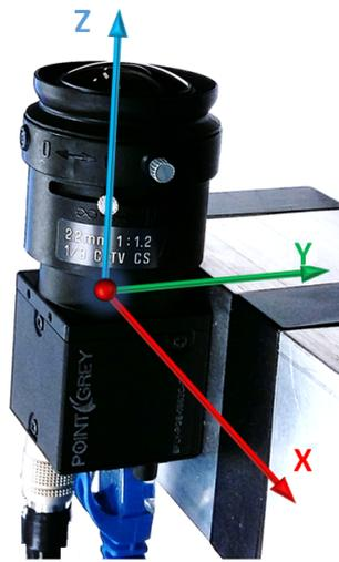
Figure 11. Upward-pointing camera coordinates system.
