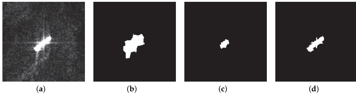
Figure 7. Detection results of one ship slice: (a) original ship slice, (b) detection result of the VWIE method, (c) detection result of the CA-CFAR method and (d) detection result of the proposed method.
