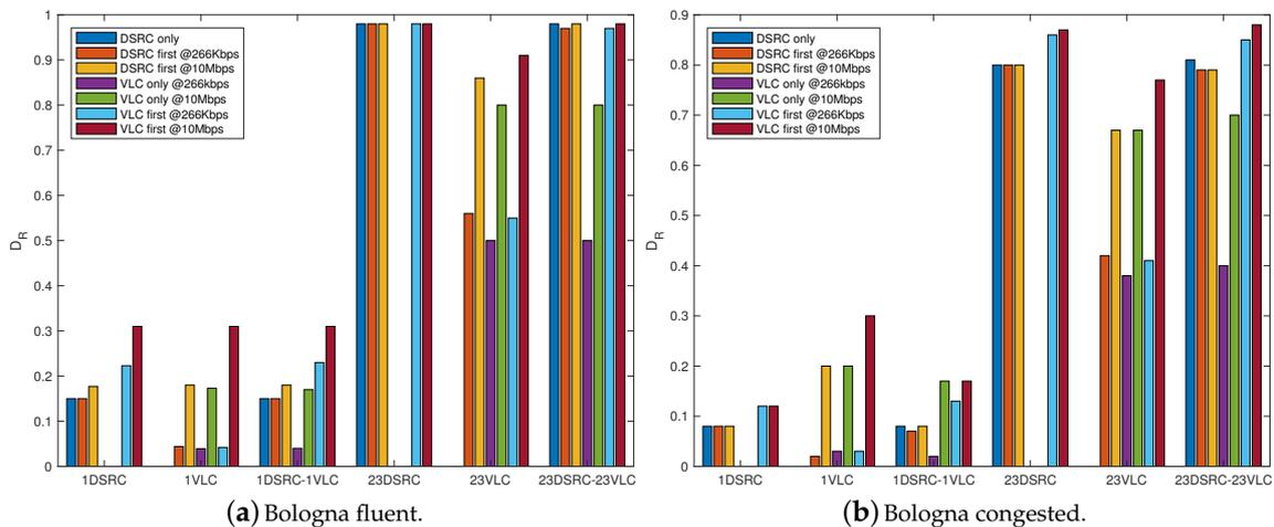
Figure 7. Delivery rate for various number of RSUs and  $\lambda = 10$  packet/s in fluent (a) and congested (b) traffic conditions.
