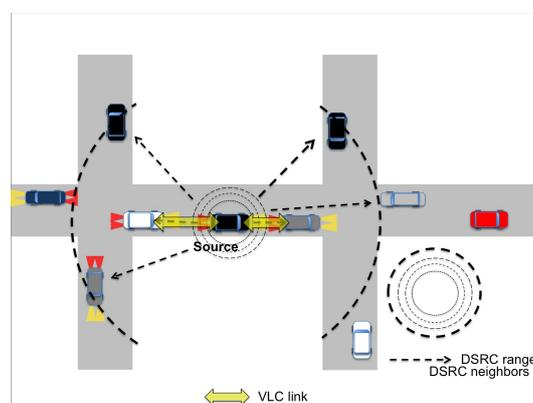
**Figure 1.** VLC and IEEE 802.11p links and coverage.
