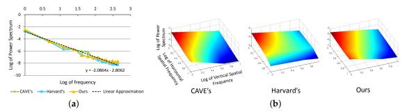
**Figure 3.** Spectral reflectance in four different data sets (Harvard's [31], CAVE [38], and our dataset) have similar behavior after Fourier transform. (a) Log of power spectrum of spectral component in four different data sets; (b) log of power spectrum of spatial component in four different data sets.
