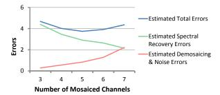
**Figure 13.** Our estimated error (spectral recovery error, demosaicing error and imaging noise) on "CAVE" spectral dataset [38] with a different number of mosaiced channels. The errors reveal the optimal number of channels to be around 5–6. Here, we use the MSFA and demosaicing method in [26].
