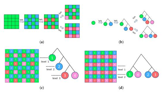
**Figure 4.** (a) Generation of the MSFAs. (b) Generation of the binary trees. (c,d) Left: two patterns of four channels MSFA; right: the binary trees of the four channels pattern have four leaves, each leaf represents a spectral channel. The four leaf nodes correspond to the four spectral channels with (c) sampling rate  $\{\frac{1}{2}, \frac{1}{4}, \frac{1}{8}, \frac{1}{8}\}$  and (d) sampling rate  $\{\frac{1}{4}, \frac{1}{4}, \frac{1}{4}, \frac{1}{4}\}$ .
