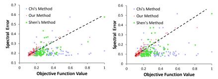
**Figure 8.** Relationship between spectral estimated error and objective function value of previous methods and our method on "natural" (**left**) and "paper" (**right**) dataset in [47]. Note the scatters of our method distribute along the black dashed line while the scatters of the previous method distribute irregularly.
