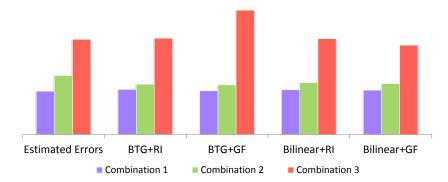
**Figure 10.** Comparison between estimated errors and actual reconstruction errors using different demosaicing methods (BTG + RI, BTG + GF, Bilinear + RI, Bilinear + GF) with the channels and patterns shown in Figure 9. The estimated errors are scaled for comparison.
