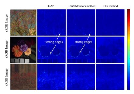
**Figure 12.** Reconstruction spectral error of multi-spectral images in our database (the 1st row), CAVE spectral database (the 2nd row), and Harvard's database (the 3th row) using a GAP camera, Chi and Monno's method and our mosaic camera (see Figure 11). Please zoom in and see sharp edges in gray images.
