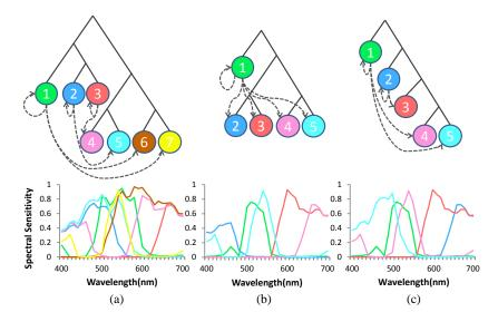
**Figure 11.** Selected channels, mosaic binary tree, and demosacking order of (a) GAP camera; (b) Chi and Monno's method; and (c) our method.
