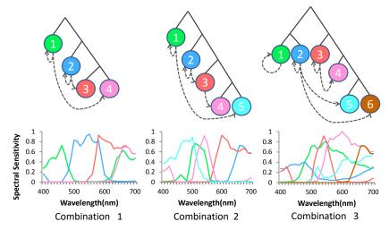
**Figure 9.** Three examples of combinations of different channels, MSFA patterns and demosaicing orders. Note that the three examples have different numbers of channels (4, 5, 6). The combinations are set casually to verify our overall model.
