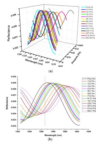
**Figure 7.** Interferograms of the zeolite film-coated FOI sensor under equilibrium states at various  $P_{isob}$ : (a) 3-D presentation and (b) 2-D view of interference evolution with equilibrium  $P_{isob}$ .
