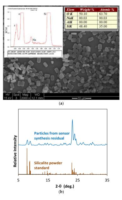
**Figure 5.** Characterizations of the crystals collected from the residual solution in the zeolite film synthesis vessel: (**a**) SEM picture with inserts showing the EDS spectrum and elemental composition and (**b**) XRD pattern in comparison with standard of silicalite powder.
