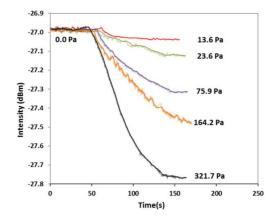
**Figure 10.** Temporal responses of reflection intensity at  $\lambda = 1566$  nm to one-step  $P_{isob}$  increase from 0 Pa to various specific values.
