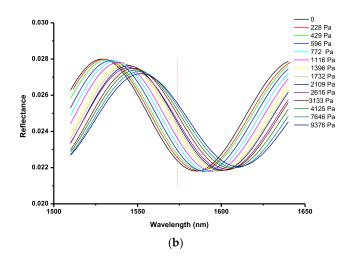
**Figure 12.** Interference spectra at 80 °C as a function of  $P_{isob}$ : (**a**) 3-D presentation and (**b**) 2-D view of interference evolution with equilibrium  $P_{isob}$ .
