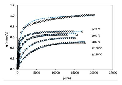
**Figure 6.** Isotherms of isobutane in silicalite at various temperatures (dashed lines are least square regressions using the extended Langmuir equation).
