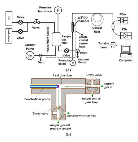
**Figure 3.** Schematics showing (**a**) the experimental system for FOI sensor operation; and (**b**) the FOI sensor head installation in the testing chamber.
