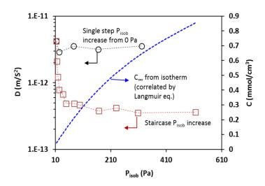
**Figure 11.** The transport diffusivity measured under the two conditions shown as a function of  $P_{isob}$  together with the corresponding isobutane equilibrium concentration in the zeolite.
