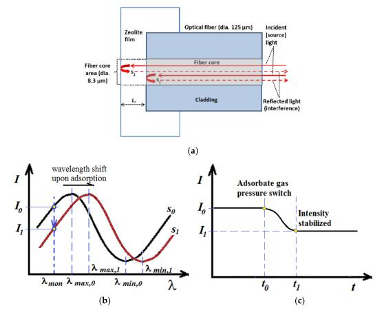
**Figure 1.** Schematics showing (**a**) the zeolite film-coated fiber optic interferometer (FOI) sensor head; (**b**) illustration of the reflected light interference spectrum shift upon adsorption; and (**c**) reflection intensity (I; signal S) as a function of time at a fixed wavelength during the dynamic process of adsorption.
