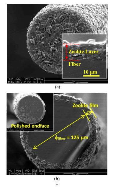
**Figure 4.** SEM pictures of the zeolite film-coated FOI sensor head: (**a**) unpolished zeolite film on fiber endface; (**b**) fracture cross-section of zeolite coating on the fiber side surface with the insert showing the endface film after polishing.
