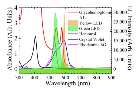
**Figure 2.** Electroluminescence of green and yellow LED measured at room temperature compared to the absorbance of Glycohemoglobin A1*c*, Hemotrol, crystal violet, and rhodamine 6 g solutions.
