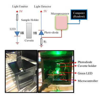
**Figure 1.** (**a**) The schematic of the experimental setup used to calibrate and test glycated hemoglobin concentration. (**b**) Snapshots of the designed prototype.
