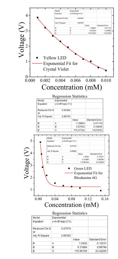
**Figure 3.** Photodiode output voltage (averaged over 500 voltage readings) as a function of concentration of (**a**) Crystal Violet synthetic dye using the yellow LED and (**b**) rhodamine 6 g fluorescent dye using the green LED. The data points are fitted to an exponentially decaying equation model via a three-variable regression analysis to find molar absorption coefficient.
