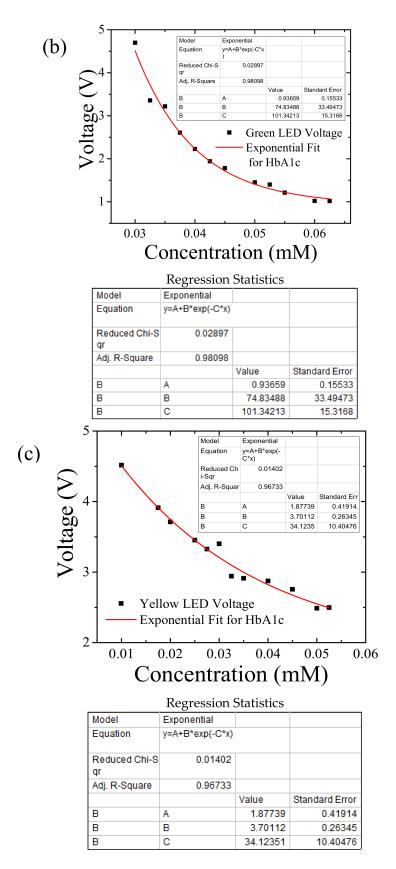
**Figure 4.** (a) The absorption spectra of diluted concentrations of glycohemoglobin A1c solutions measured at room-temperature. (b) Photodiode output voltage (averaged over 500 voltage readings) as a function of concentration for diluted concentrations of glycated hemoglobin using green LED and (c) yellow LED. The data points are fitted to an exponentially decaying equation using a three-variable regression analysis.
