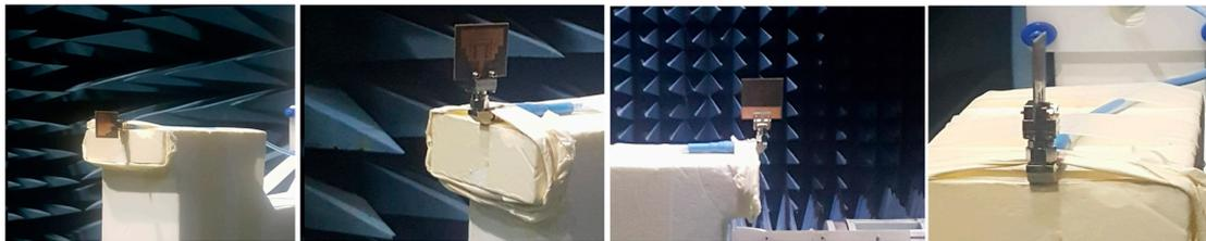
**Figure 10.** Radiation pattern measurement setup for the reference and proposed antenna at different orientations in the anechoic chamber.
