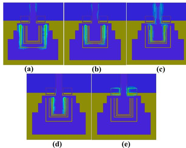
**Figure 6.** Surface current distributions of the proposed antenna at the corresponding center frequencies of the notched bands (a) 3.5 GHz; (b) 4.5 GHz; (c) 5.25 GHz; (d) 5.7 GHz; (e) 8.2 GHz.
