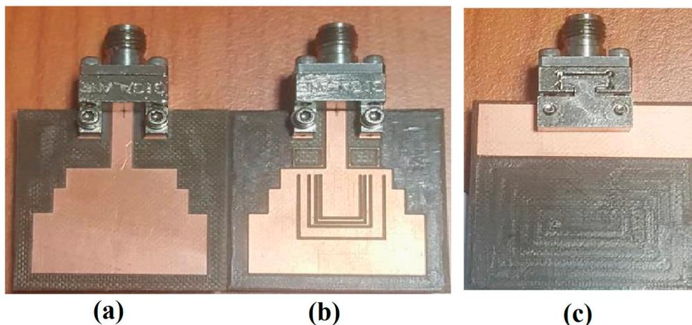
**Figure 2.** Prototype of the reference and proposed antenna. (a) The reference antenna (front view); (b) the proposed antenna (front view); and (c) the reference and proposed antenna (rear view).
