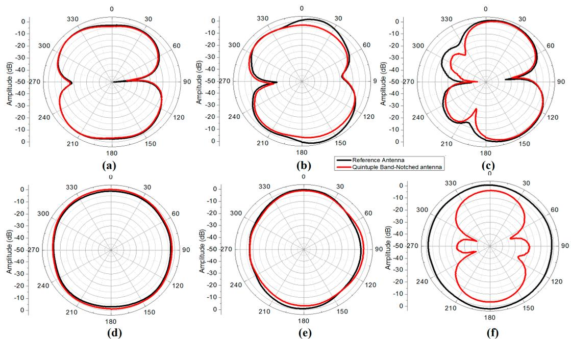
**Figure 11.** Measured radiation patterns of the reference vs. quintuple band-notched antenna (a) XZ plane (3.9 GHz); (b) XZ plane (6.1 GHz); (c) XZ plane (7.8 GHz); (d) YZ plane (3.9 GHz); (e) YZ plane (6.1 GHz); (f) YZ plane (7.8 GHz).
