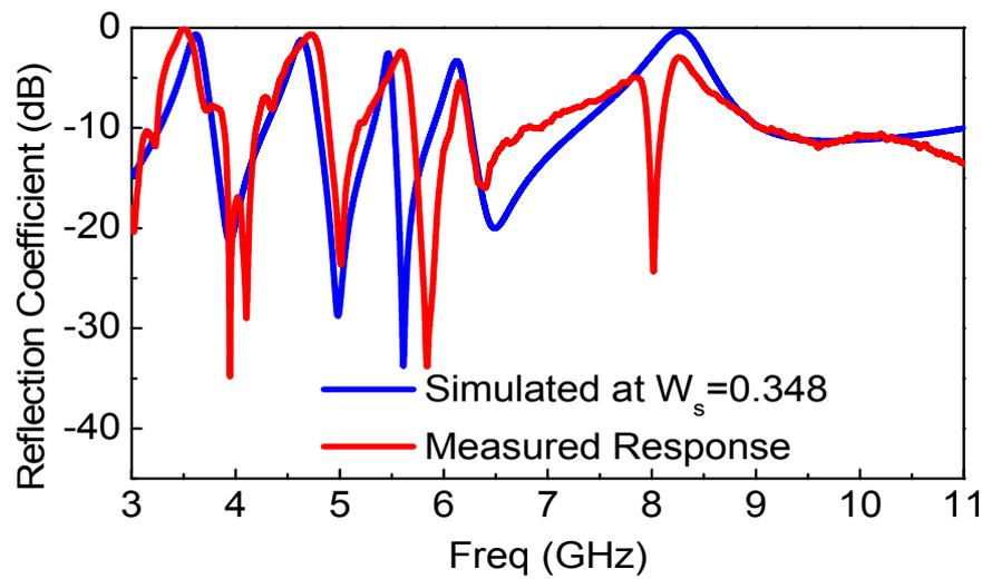
**Figure 9.** Simulated vs. measured frequency response of the proposed quintuple band-notched UWB antenna when  $W_s = 0.348$  mm in the simulation setup.
