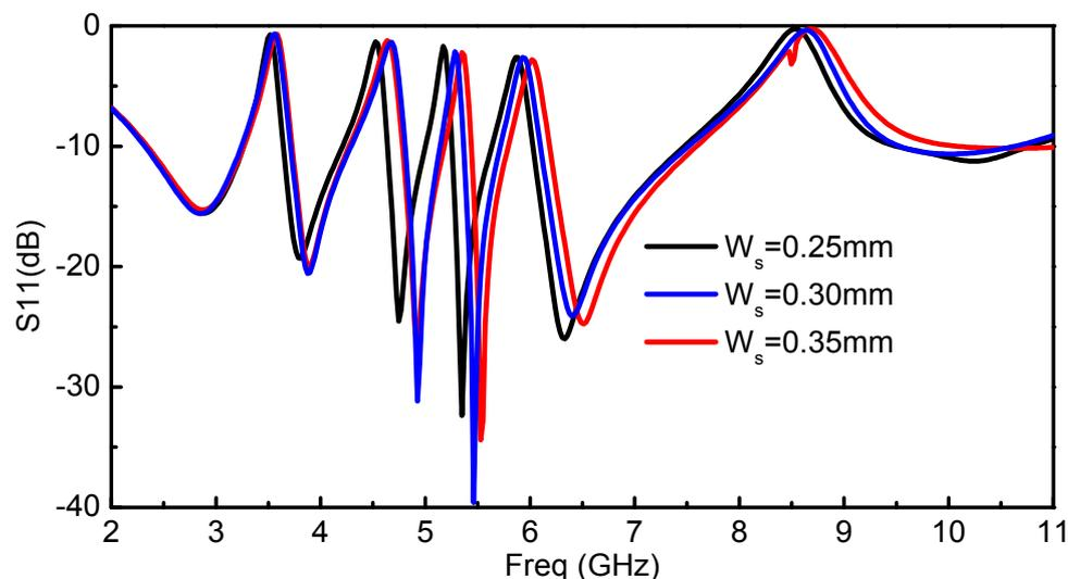
Figure 7. Effect of critical parameter  $W_s$  on the response of the proposed antenna.
