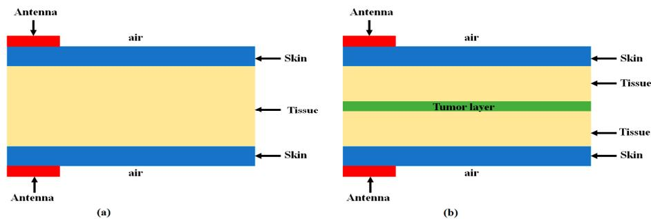
**Figure 12.** Breast phantom model developed for investigation of tumor cell (cross view). (a) Breast phantom without tumor; (b) Breast phantom with tumor.
