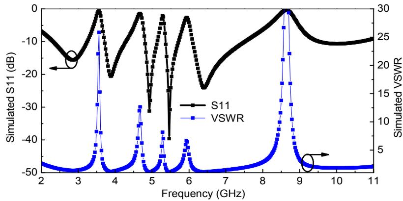
**Figure 4.** Simulated reflection coefficient and VSWR (Voltage Standing Wave Ratio) of the proposed quintuple band-notched UWB antenna.
