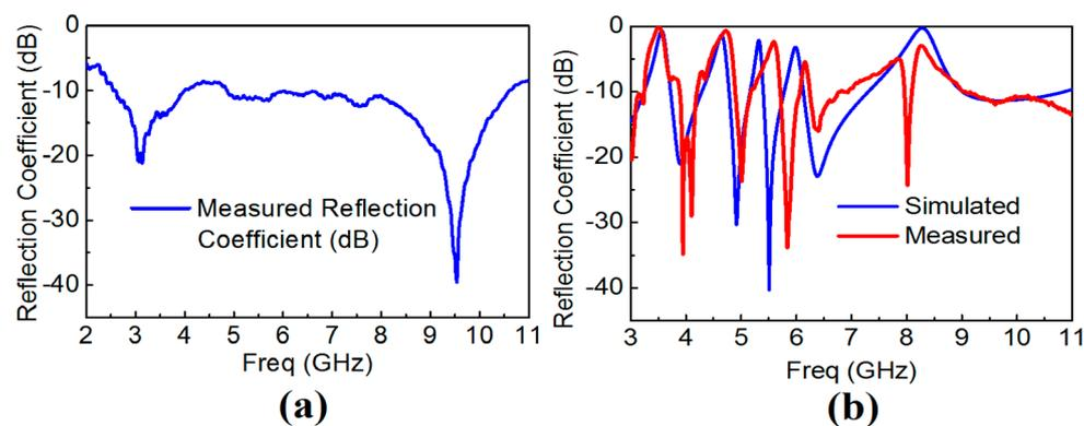
**Figure 8.** The measured frequency response of the reference and proposed quintuple band-notched UWB antenna (a) Measured reflection coefficient of the reference antenna; (b) Measured vs. simulated reflection coefficient of the proposed quintuple band-notched antenna.
