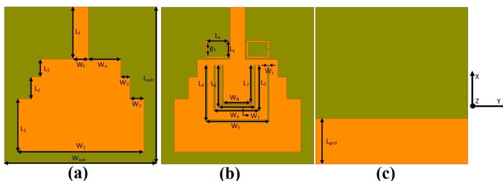
**Figure 1.** The geometry of (a) the reference antenna (front view); (b) the proposed antenna (front view); and (c) the reference and proposed antenna (rear view).
