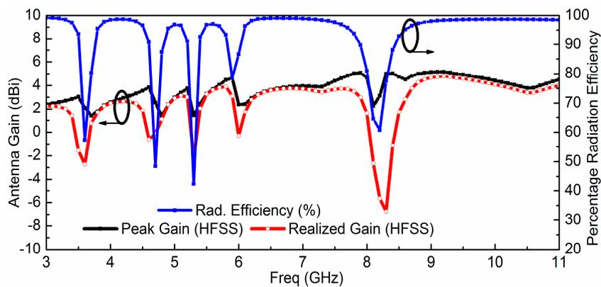
**Figure 5.** Simulated antenna gain from the radiator, percentage radiation efficiency, and realized antenna gain including the effects of the input mismatch of the quintuple band-notched UWB antenna.
