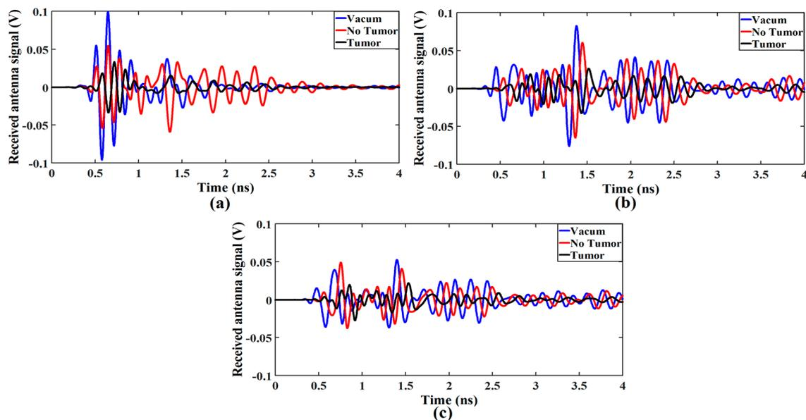
**Figure 13.** Received waveform responses for (a) Both antennas are placed in contact with stacked organic layers, and each antenna is placed (b) 5 mm away and (c) 10 mm from the stacked organic layers.
