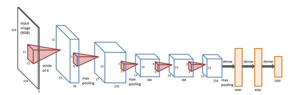
Figure 2. An illustration of the architecture of the DCNNs proposed by Alex et al. [30].
