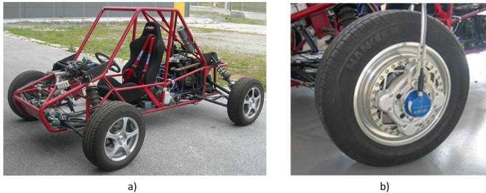
Figure 1. (a) IMMa sensorized vehicle. (b) Detail of the measuring rim.
