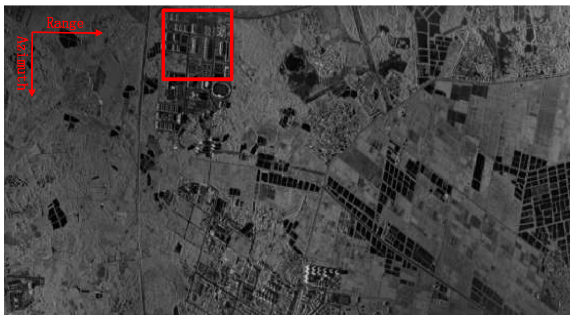
Figure 3. First processed sliding spotlight SAR image via the proposed approach.
