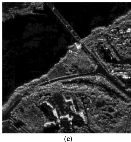
Figure 8. A typical area in Figure 6 are zoomed and compared with the other methods. (a) Focused without MOCO; (b) Focused with only range-varying PGA; (c) Focused combining stripmap RDM and range-varying PGA; (d) Focused combining sliding spotlight RDM without WTLS and range-varying PGA; (e) Focused combining sliding spotlight RDM with WTLS and range-varying PGA.
