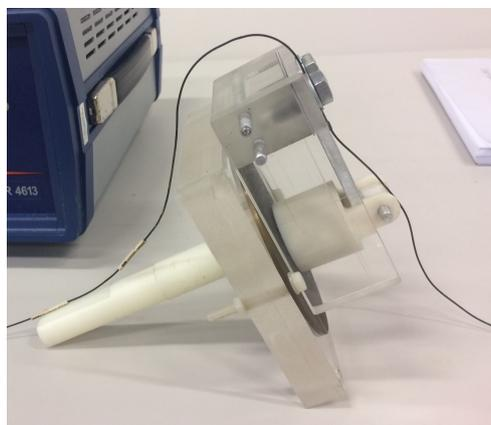
**Figure 11.** Fixture comprised of an acrylic plate and a nylon rod holds the steel disc with a sensor prototype.
