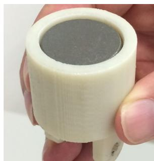
**Figure 9.** 1 mm gap left in magnet cover.
