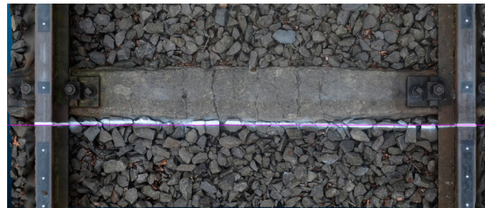
Figure 9. Generated 3D model of railway track with simulated structured light (SSL) profile.
