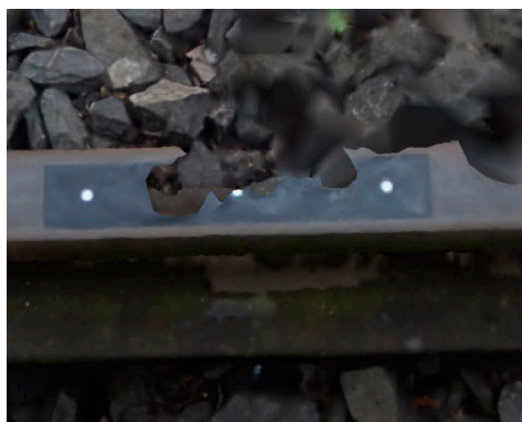
Figure 7. Holes on control points (CrIP) triplet in the 3D mesh model generated by RealityCapture software.
