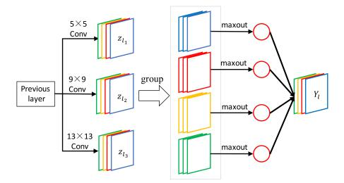
Figure 3. The proposed module which produces the maxout results of multi-scale convolutional.
