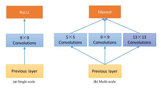
**Figure 1.** The single scale convolutional layer and the proposed multi-scale competitive module are depicted in (**a**) and (**b**), where (**a**) only contains single scale convolutional filters within each module, whereas (**b**) contains three scale of convolutional kernel.
