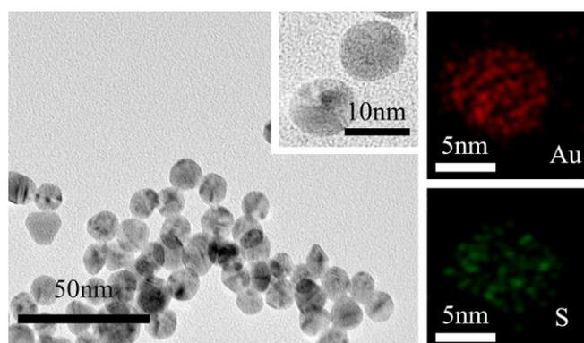
**Figure 2.** TEM images and energy dispersive spectrometry (EDS) element mappings of the  $\beta$ -CD@AuNPs; the red and green colors correspond to elemental Au and S, respectively.
