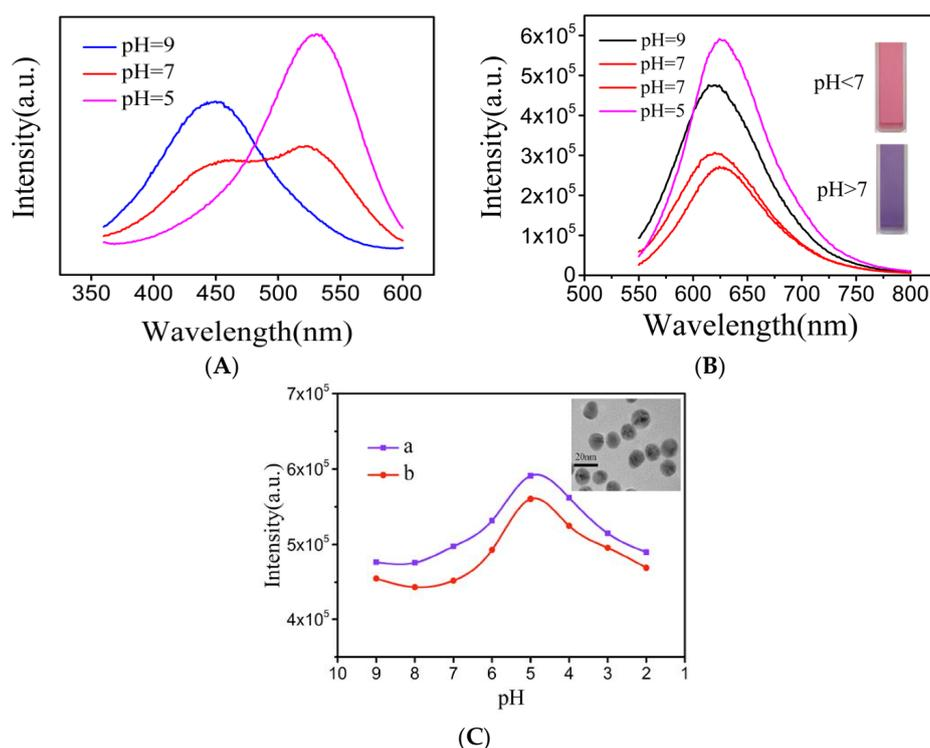
**Figure 4.** (A) Excitation spectra of the NR- $\beta$ -CD@AuNPs at pH values of 9, 7, and 5; (B) Emission spectra of the NR- $\beta$ -CD@AuNPs at pH values of 9, 7, and 5; (C) Fluorescence intensity of the NR- $\beta$ -CD@AuNPs (a) and the NR- $\beta$ -CD@AuNPs in the presence of  $NO_2^-$  ( $100 \mu\text{g}\cdot\text{L}^{-1}$ ) (b); Inserted image: TEM image of the NR- $\beta$ -CD@AuNPs at a pH value of 5.
