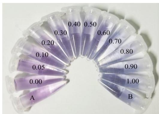
**Figure 6.** Photograph of the NR- $\beta$ -CD@AuNPs in the presence of different  $[\text{NO}_2^-]$  concentrations including 0, 0.05, 0.10, 0.20, 0.30, 0.40, 0.50, 0.60, 0.70, 0.80, 0.90, and  $1.00\ \mu\text{g}\cdot\text{mL}^{-1}$ ; A:  $0\ \mu\text{g}\cdot\text{mL}^{-1}$  of  $[\text{NO}_2^-]$  and competing ions; and B:  $1.00\ \mu\text{g}\cdot\text{mL}^{-1}$  of  $[\text{NO}_2^-]$  and competing ions.
