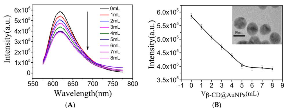
**Figure 3.** (A) Fluorescence spectra of the NR- $\beta$ -CD@AuNPs when the volume of  $\beta$ -CD@AuNPs was 1, 2, 3, 4, 5, 6, 7, and 8 mL. (B) Plots of the NR- $\beta$ -CD@AuNPs fluorescence intensities versus the volume of the  $\beta$ -CD@AuNPs with error bars. Inserted image: TEM image of the NR- $\beta$ -CD@AuNPs.
