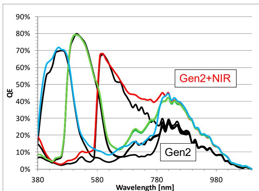
**Figure 10.** QE comparison from a  $1\ \mu\text{m}$ , 16MP Gen2 image sensor to one with an additional process for NIR enhancement.
