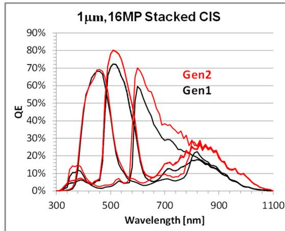
Figure 4. QE comparing Gen1 and Gen2 1  $\mu\text{m}$ , 16 MP technologies.
