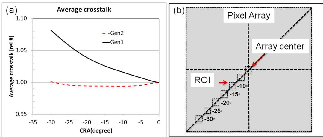
Figure 5. (a) Crosstalk vs angle, calculated from QE curves measured in a fix ROI along a diagonal as shown in the (b). Angles are the CRA of the module lens at each ROI.
