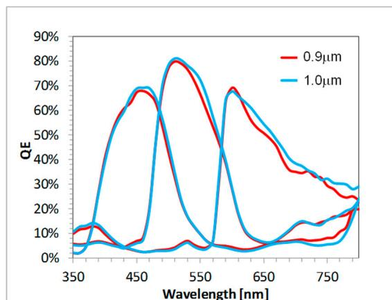
Figure 6. The QE from 1  $\mu\text{m}$  and 0.9  $\mu\text{m}$  pixel products, both using the Gen2 BSI-stacking technology.
