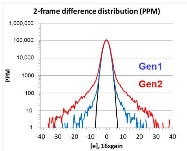
**Figure 8.** Two-frame difference image, noise histogram comparing the 1  $\mu\text{m}$ , 16 MP images sensors that use the Gen1 and Gen2 technology.
