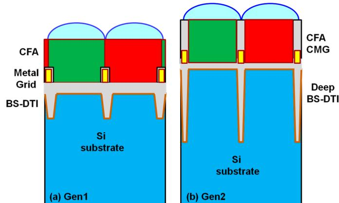
Figure 3. Gen1 (a) and Gen2 (b) schematic; Gen2 BSI stack has thicker silicon, narrower and deeper BS-DTI, and a composite metal-oxide, back-side grid.
