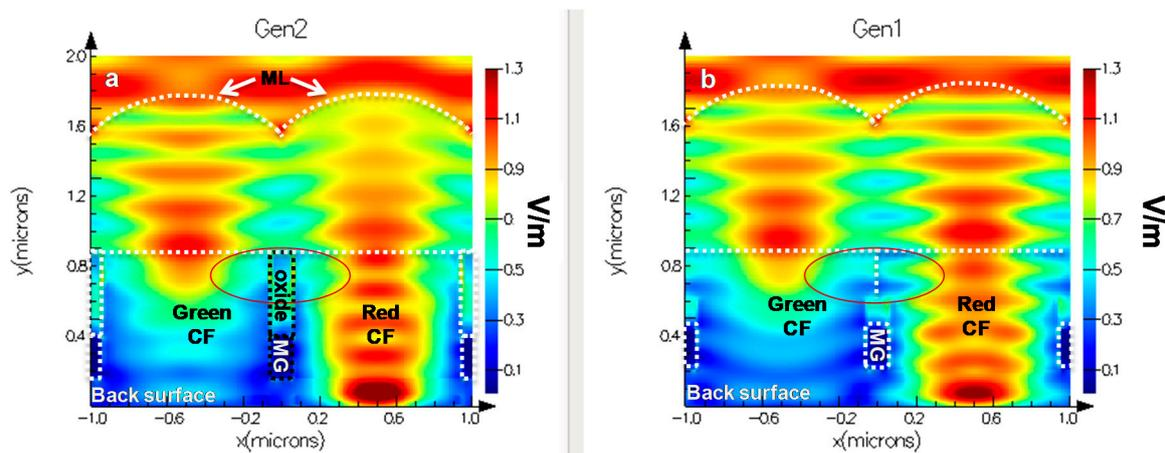
**Figure 7.** FDTD simulation comparing the light confinement of Gen2 (left) and Gen1 (right). Simulations used a monochromatic plan wave at, 630 nm TE mode, incident on the Green and Red pixel of each structure. Structure features are labeled and highlighted.
