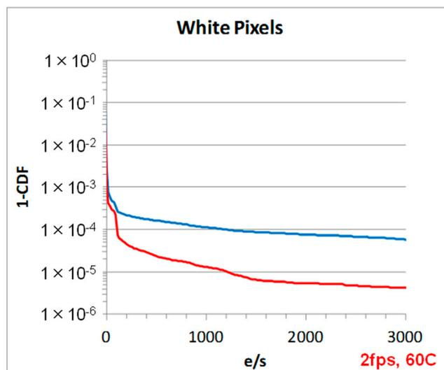
**Figure 9.** Plot of 1-cumulative density function (1-CDF) comparing the dark image from low white-pixel, PD process. 1  $\mu\text{m}$ , 16 MP (2 fps, 60 C).
