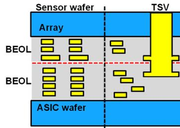
Figure 1. First-generation BSI-CIS stacking with oxide-oxide bonding and TSV.
