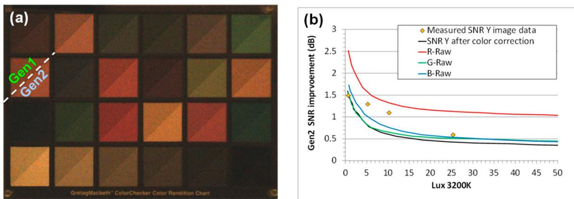
**Figure 11.** (a) Combined Macbeth chart images from 16 MP, 1  $\mu\text{m}$  pixel Gen1 and Gen2 products to show the Gen2 low light (5 Lux) sensitivity improvement. (b) Gen2 SNR improvement vs. lux level, including measured data and simulated results (F2.0, 15 fps).
