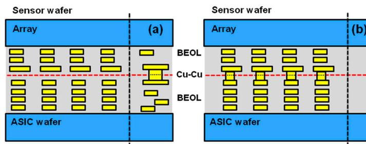
Figure 2. Hybrid bond-stacking schematic, showing the Cu-Cu interconnects outside the array (a) and within the array (b).
