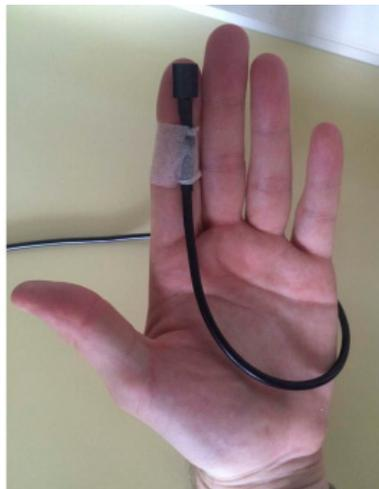
**Figure 7.** Response button used for answering to Detection-response task (DRT) stimuli [24].
