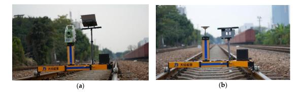
**Figure 8.** Modular design of the TGMT based on aided INS. (**a**) TGMT with TS/INS configuration; (**b**) TGMT with GNSS/INS configuration.
