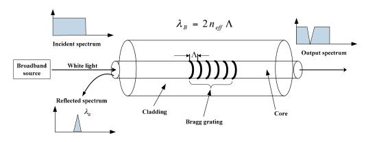
Figure 1. Measurement principle of FBG sensor.
