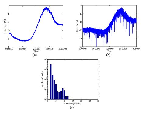
**Figure 7.** Raw data of selected FBG sensors during bridge operation phase on 29 December 2015: (a) Temperature time history measured by FBG-MS-NT-2; (b) Stress time history measured by FBG-MS-NS-2-3; (c) Histogram of daily stress spectrum.
