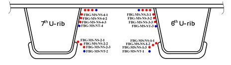
Figure 3. Deployment of FBG sensors.
