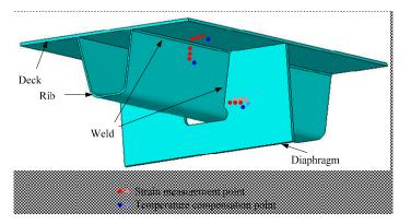
Figure 5. Details of measurement points.
