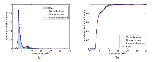
Figure 11. Distribution function of stress range: (a) Finite mixture PDFs; (b) Finite mixture CDFs.
