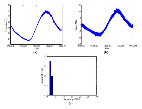
**Figure 6.** Raw data of selected FBG sensors during bridge construction phase on 17 October 2015: (a) Temperature time history measured by FBG-MS-NT-2; (b) Stress time history measured by FBG-MS-NS-2-3; (c) Histogram of daily stress spectrum.
