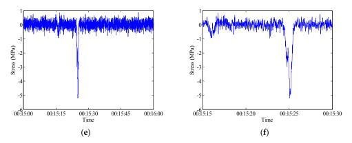
**Figure 8.** Raw data measured by FBG-MS-NS-2-3: (**a**) Stress time history; (**b**) Temperature time history; (**c**) Live-load induced stress time history in 1 h; (**e**) Live-load induced stress time history in 1 h; (**e**) Live-load induced stress time history in 1 s.
