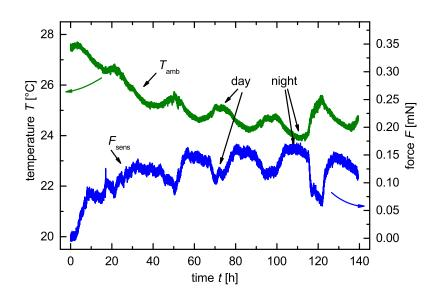
**Figure 3.** Fluctuating ambient temperature  $T_{amb}$  in the laboratory and the inverse proportional measured force *F* over a time period of  $\Delta t = 140$  h.
