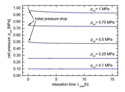
**Figure 4.** Mechanical relaxation of the pressure monitoring cell for  $p_{init} = 0.1$  MPa, 0.25 MPa, 0.5 MPa, 0.75 MPa and 1 MPa. An increasing initial pressure leads to an increasing relaxation time  $t_{relax}$  and a higher initial pressure drop.
