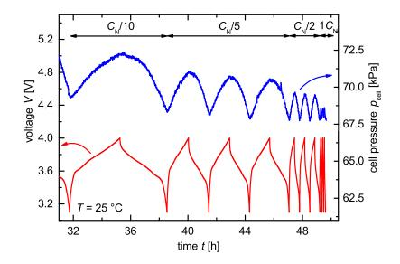
**Figure 5.** Pressure-time and voltage-time curves of a constrained NCM/graphite coin cell at several C-rates using a pressure monitoring cell for constrained battery electrodes. The cell pressure  $p_{cell}$  correlates with the voltage *V* of the electrochemical cell. The pressure difference during cycling decreases with increasing current.
