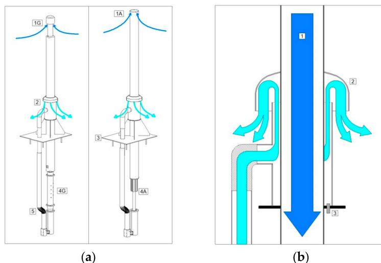
**Figure 1.** (a): air intake systems for RGs (left) and AEs (right). The numbers in the technical diagram denote: air inlet (1), air exhausts (2), flanges for mounting on the roof (3), manifolds for the connection of tubing to analyzers (4), high-velocity fan (5). (b): details of the air streams in the proximity of the air exhaust. Dark and light arrows represent the air stream at the inlet and at the exhaust of the intakes, respectively.
