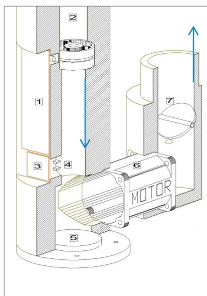
**Figure 2.** Diagram of the flow generator and control systems: flow control board (1), anemometer (2), T and RH control board (3), T and RH sensor (4), water drainage (5), motor and fan (6), manual air flow shutter (7). The arrows denote the flow direction.
