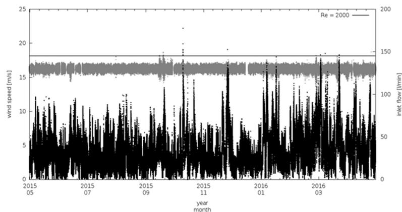
**Figure 7.** Time series of sampling flow of the aerosol intake (grey) and wind speed (back) at CGR (1-min averages). The top black straight line represents the maximum allowed flux to maintain a laminar regime in the aerosol air intake.
