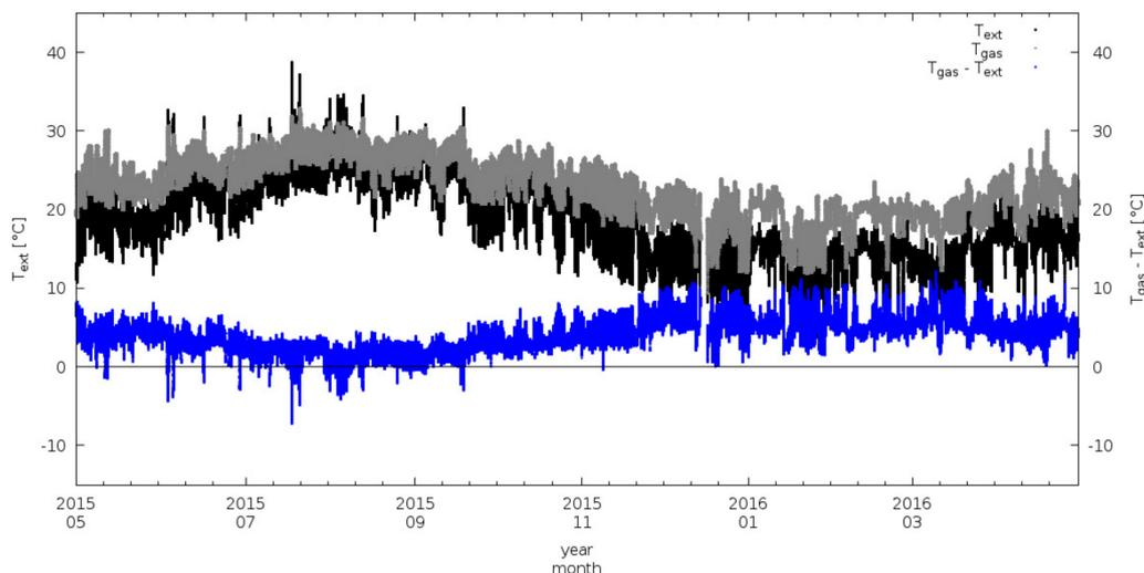
**Figure 10.** Time series of ambient air temperature ( $T_{ext}$ , black), internal temperature of gas intake ( $T_{gas}$ , grey) and their differences ( $T_{gas}-T_{ext}$ , blue). 1-min average values are reported.
