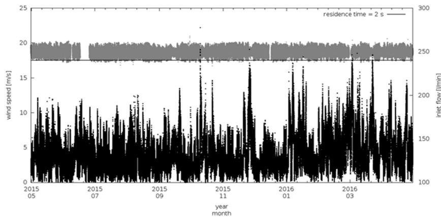
**Figure 6.** Time series of sampling flow of trace gas intake (grey) and wind speed (back) at CGR (1-min averages). The top black straight line represents the minimum allowed flux to maintain the air residence time below 2 s in the air intake.
