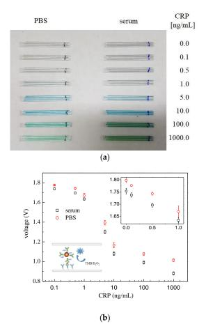
**Figure 5.** (a) Picture of the capillary tubes that had undergone "AuNP capillary ELISA" either under PBS or serum, and (b) their logarithmic plot of optical density expressed in voltage against CRP concentration with the inset representing linear plot in the lower concentration range.
