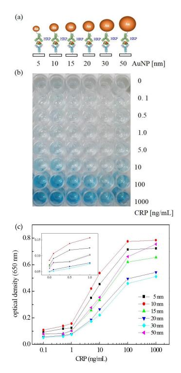
**Figure 1.** (a) The schematic view of the sandwich ELISA using AuNP•antiCRP-HRP with varying diameters of the AuNPs involved, (b) the picture of 96-well plate of the resulting ELISA produced based on the AuNP•antiCRP-HRPs, and (c) the plot of optical density and CRP concentration for the "AuNP ELISA" with varying diameter of AuNPs.
