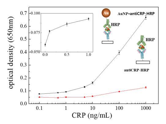
**Figure 3.** Logarithmic plots of optical density against CRP concentration of the "AuNP ELISA" (AuNP 10 nm) (black line) and the conventional ELISA (red line) with the inset representing the linear plot of the lower concentration range of the "AuNP ELISA".
