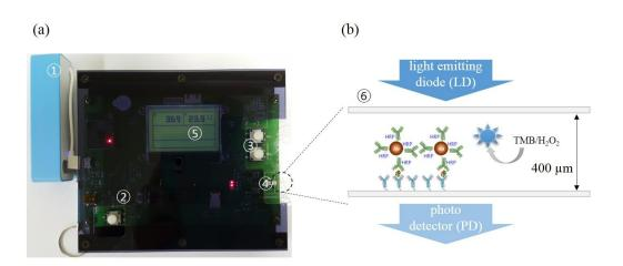
battery, 2. power button, 3. display brightness controller,
