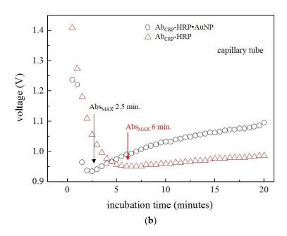
**Figure 7.** Plots representing the monitoring of the ELISAs either on (**a**) the 96-well plate, or (**b**) the capillary tube using AuNP•antiCRP-HRP (black circle) and antiCRP-HRP (red triangle) as indicator antibodies.
