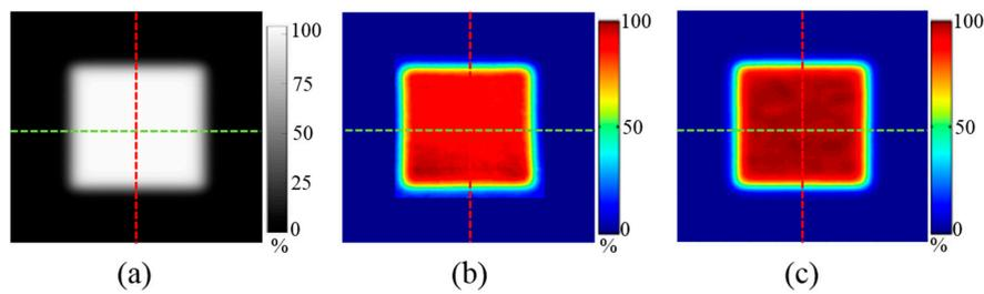
**Figure 4.** An example of measured 2D dose distributions using various dosimetric tools (Case 3 of the square-shaped field in Table 1). (a) MatriXX; (b) EBT3 film; (c) FORS.
