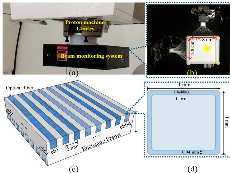
**Figure 2.** (a) Configuration of the developed FORS based proton beam dosimetry system; (b) The inside view of the developed proton beam dosimetry system; (c) Schematic image of the side-view of the FORS; (d) Schematic image of cross-section of the optical fiber.
