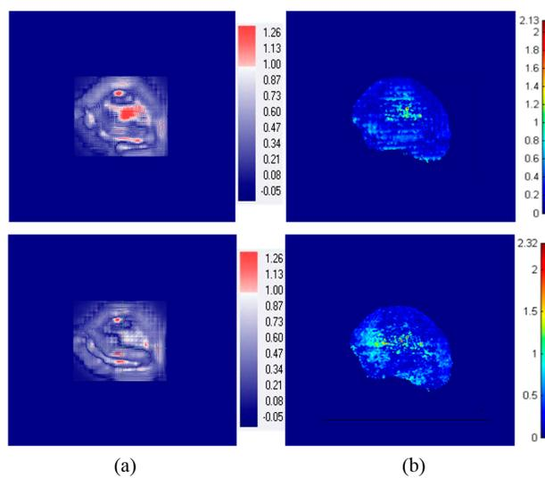
**Figure 6.** Example of dose comparison using the gamma evaluation method for an irregularly-shaped field. (Field 5 in Table 2). (a) MatriXX vs. FOR; (b) EBT3 film vs. FORS. The number denotes the gamma index.
