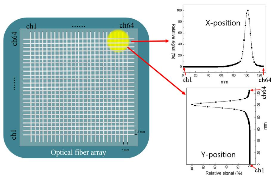
**Figure 3.** Schematic image of position localization using the FORS.
