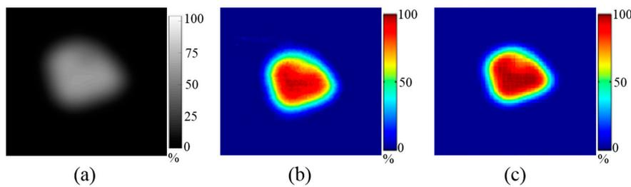
**Figure 5.** An example of measured 2D dose distribution using various dosimetric tools for the irregular-shaped field. (Field 4 in Table 2) (a) MatriXX; (b) EBT3 film; (c) FORS.
