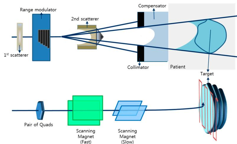
**Figure 1.** Proton beam delivery techniques: Passive scattering mode (**upper panel**) and Pencil beam scanning mode (**lower panel**).
