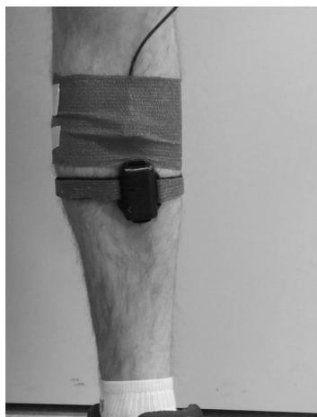
**Figure 3.** Attachment method of the IMU and the reference sensor on the subject's leg.
