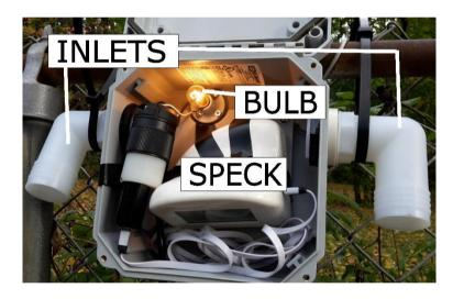
Figure S1. Inside of outdoor housing for Speck monitor with labeled inlets, Speck monitor, and a bulb for heating.
