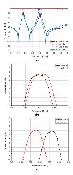
**Figure 7.** (**a**) Measured S-parameters of the proposed filter without and with EGaIn and insertion loss without and with EGaIn (**b**) in odd mode; and (**c**) in even mode.
