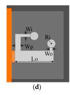
**Figure 1.** Top view of the proposed filter: (**a**) using two split-ring resonators (SRR); (**b**) with stub; (**c**) with stub and microfluidic channel; and (**d**) an enlarged top view of the microfluidic channel.
