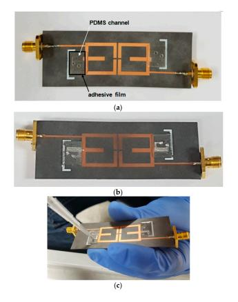
**Figure 6.** Pictures of the fabricated proposed filter: (**a**) without EGaIn; (**b**) with EGaIn; and (**c**) in the process of injecting EGaIn.
