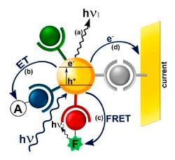
**Figure 2.** Schematic representation of different QD-based sensing configurations [26]. (**a**) luminescence, (**b**) electron transfer, ET, (**c**) Förster resonance energy transfer, FRET, or (**d**) photocurrent generation.
