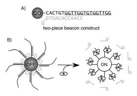
**Figure 3.** Design of a QD aptamer beacon for the detection of thrombin. (**A**) Anti-thrombin aptamer sequence (black) and quench oligonucleotide (gray). (**B**) Schematic for detection [48].
