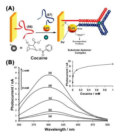
**Figure 7.** (**A**) Photoelectrochemical cocaine sensor with the self-organization of cocaine/aptamer subunits on an Au electrode. (**B**) Photocurrent action spectra with the analysis of different concentrations of cocaine [46].
