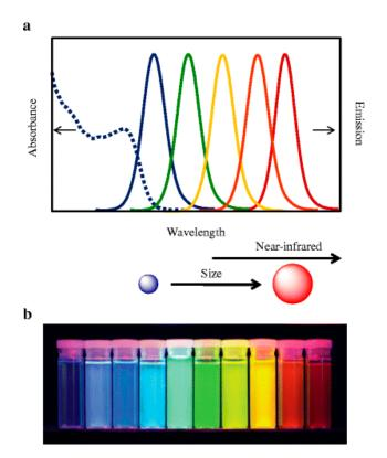
**Figure 1.** (a) Size-tunable emission spectra of QDs; (b) 10 distinguishable emission colors of ZnS-capped CdSe QDs by a near-UV lamp. From left to right (blue to red), the emission maxima are located at 443, 473, 481, 500, 518, 543, 565, 587, 610, and 655 nm [6].
