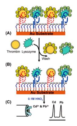
**Figure 6.** Operation of the aptamer/QD-based dual-analyte biosensor, through displacement of the tagged proteins with the target analytes. (**A**) Monolayer of thiolated aptamers is mixed with the bound protein-QD conjugates; (**B**) The tagged proteins is displaced by the sample; (**C**) The remaining captured nanocrystals are dissolved and apply their electrochemical-stripping detection [43].
