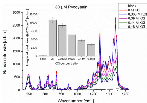
**Figure S3.** Mean SERS spectra of 30 μM PYO with different concentrations of KCl measured in the microfluidic platform. In the inset the integrated peak area of the PYO Raman mode at 676 cm<sup>-1</sup> and
