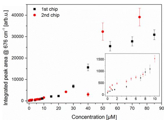
**Figure S6.** The peak area of the 676  $\text{cm}^{-1}$  Raman mode as a function of PYO concentration for 2 different chips. In the inset zoomed area for concentrations till 10  $\mu\text{M}$ .
