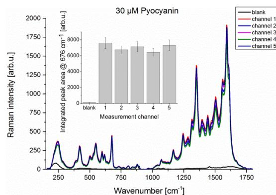
**Figure S4.** Mean SERS spectra of 30 μM PYO measured in different channels of the microfluidic chip. In the inset the integrated peak area of the PYO Raman mode at 676 cm<sup>-1</sup> and its double standard deviation is illustrated.
