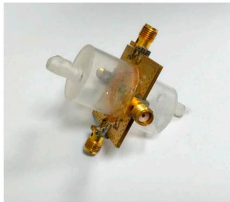
**Figure S4.** Assembled PSBAR evaluation board. The PSBAR sensing array is wire-bonded onto the evaluation board to connect vector network analyzer through SMA connectors. Plastic chambers are used to make the VOCs thoroughly contact the sensors.
