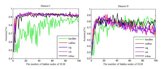
**Figure 2.** The classification accuracy of ELM in terms of 1–100 hidden nodes. The different colors of lines represent different activation functions. (Note: ELM represents the kernel extreme learning machine).
