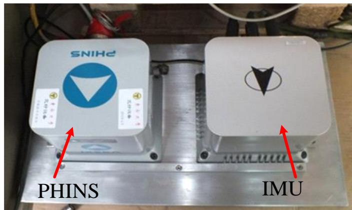
Figure 5. Installation method of the fiber optic gyro inertial system (FOSN) and the high-precision fiber optic system SINS (PHINS).
