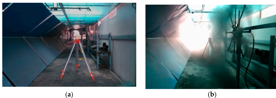
Figure 10. The experiment at gateroads of different dust concentration: (a) no coal dust; (b) a high level of coal dust.
