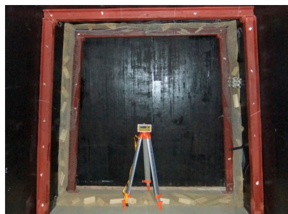
Figure 5. The surface flatness experiment of gateroads with developed deformation monitoring system.
