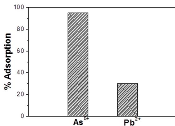
**Figure S4.** Adsorption of 10 mg GNP@Fe<sub>2</sub>CuO<sub>4</sub> composite toward 3 mg/L of As<sup>5+</sup> and Pb<sup>2+</sup> for 2 h.
