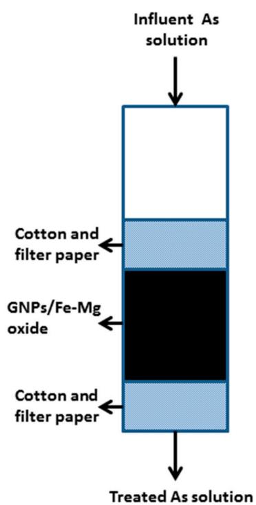
**Figure S5.** Filter column with a diameter of 2 cm and a height of 10 cm for recyclability.
