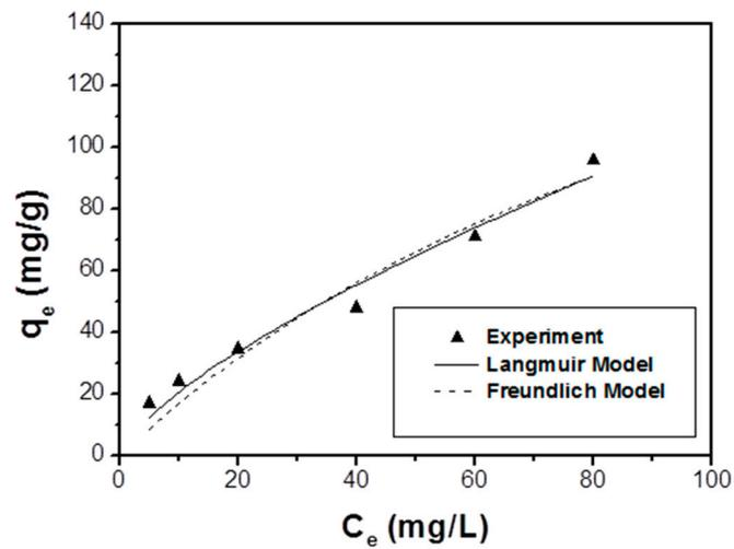
Figure S3. Adsorption isotherm for As(III) by GNP/CuFe<sub>2</sub>O<sub>4</sub> composite.
