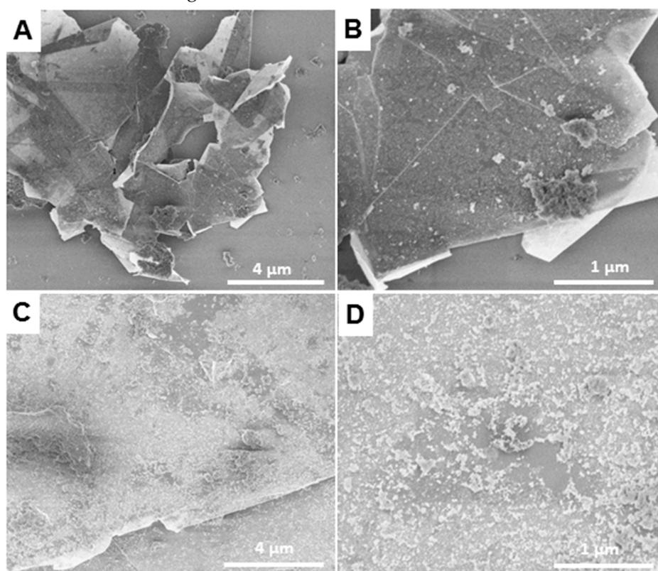
**Figure S1.** (A–D) low and high resolution SEM images of the GNPs/ $\text{CuFe}_2\text{O}_4$  composite, respectively.
