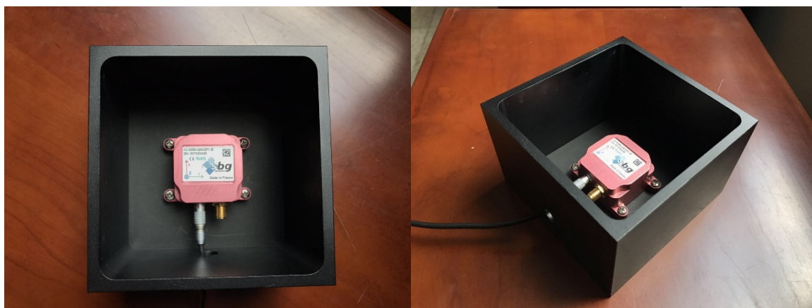
Figure 9. Cuboid frame with the mounted sensor set.
