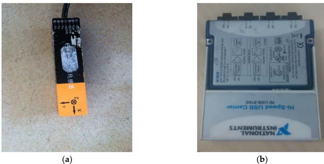
Figure 9. (a) Three-component fluxgate sensor of HS-MS-FG-3-LN; (b) Data acquisition card of NI 9239.
